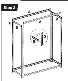
Fix Brackets 'A' to the top of Legs 'D' as shown followed by Brackets 'B'. A rubber mallet can be used to lightly tap all brackets into the keyholes of the leas.
