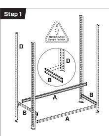
Add Foot End Caps to bottom of Legs 'D'. Fix Brackets 'A' to the bottom of Legs 'C' as shown followed by Brackets 'B'. A rubber mallet can be used to lightly tap all brackets into the keyholes of the legs. Allow one keyhole free between the foot end cap and the shelving bracket.
