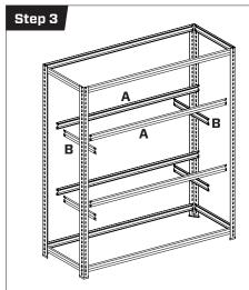
Fix remaining Brackets 'A' and Brackets 'B' to desired shelf height. As before, a rubber mallet can be used to lightly tap all brackets into the keyholes of the legs.
