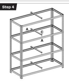
Slot Braces 'C' into position through the holes provided on Brackets 'A'.
