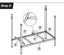
Place side brackets 'E' as shown in the diagram, followed by braces 'F' as shown
