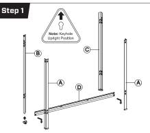
Place foot end caps onto the bottom of the legs 'A', 'B' and 'C'. Note upright position. Place shelving brackets 'D' onto the legs. A rubber mallet can be used to lightly tap all brackets into the keyholes of the legs.
