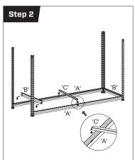
Use shelf bracket 'B' for the side brackets using the shelf bracket from Step 1 as a guide for height. Allow 1 keyhole free from the ground as shown in the diagram. Use same shelving brackets for opposing sides as shown in the diagram. Place brace 'C' as shown.
