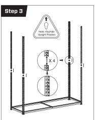
Place MDF board on bottom shelf to minimise buckling. Join the upper legs to the lower legs with the connector pins. Note upright position. Note: The legs are designed to sit directly on top of each other – don't overlap them. Handy Hint: Flathead screwdriver may be used to tap in connector pins.
