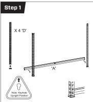
Allow one keyhole free between the foot cap and the shelving bracket.
