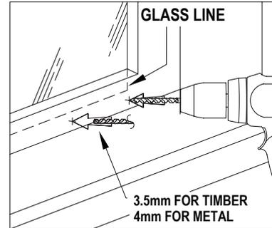
Hold Multibolt window lock in the desired position and mark the centre of the 2 x installation holes. Using a hole punch or a nail, punch the centre of the holes before drilling to make sure drill bit doesn't move. Drill 2 x 4mm holes for metal windows, 2 x 3.5mm holes windows or 2 x 3.5mm holes for timber windows at marked positions.
