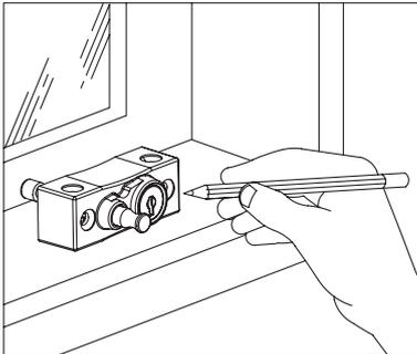
Determine the type of window you will be installing to. Make sure you choose the best fixing location for your window type. Accuracy is vital so mark and measure carefully, and drill holes level.
